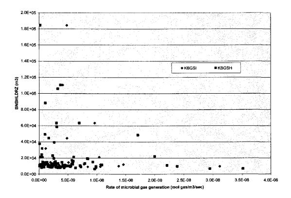
Figure 1. Plot of cumulative inflow of brine  $(m^3)$  into the repository from the Castile brine pocket BNBHLDRZ at 10,000 years versus the microbial gas-generation rates in (moles gas/m<sup>3</sup> sec). Here KBGSI is the inundated gas-generation rate and KBGSH is the humid rate.
